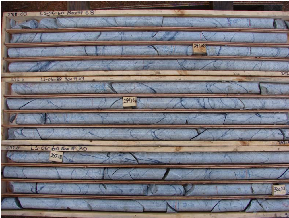
Figure 3: Drill core from Lucky Ship showing at least two phases of molybdenum mineralisation. The narrow cross-cutting veinlets show one phase and the less abundant banded vein, seen in the fourth row from the top, a second. Photograph courtesy of the company.
