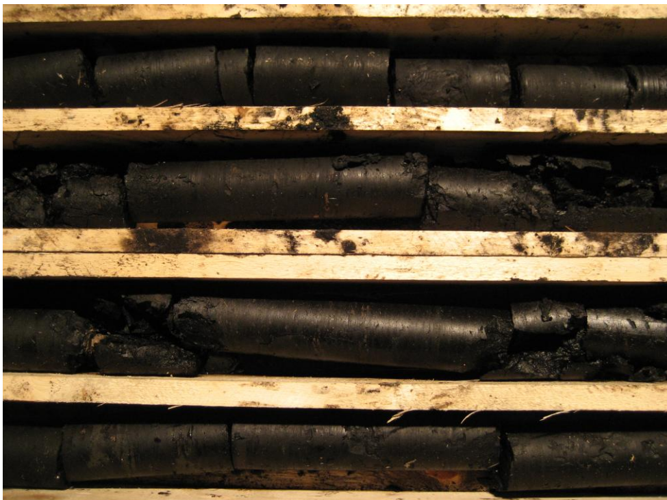
Figure 2: Close up of Leif sub-basin coal intersection with clear bright sections probably indicating higher coal rank. Source Saturn Minerals Inc
