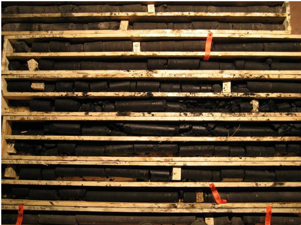
Figure 1: Core taken from the Leif sub-basin showing a 10.35m intersection. Source – Saturn Minerals Inc
