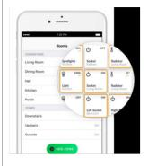
The LightwaveRF devices can be grouped by room so that a number of light switches and sockets are activated by the press of a single button on the app, or increasingly commonly, with a voice instruction to, say, Amazon Alexa to turn on or off the living room lights. Any devices can be included as well as thermostatic heating controls.
