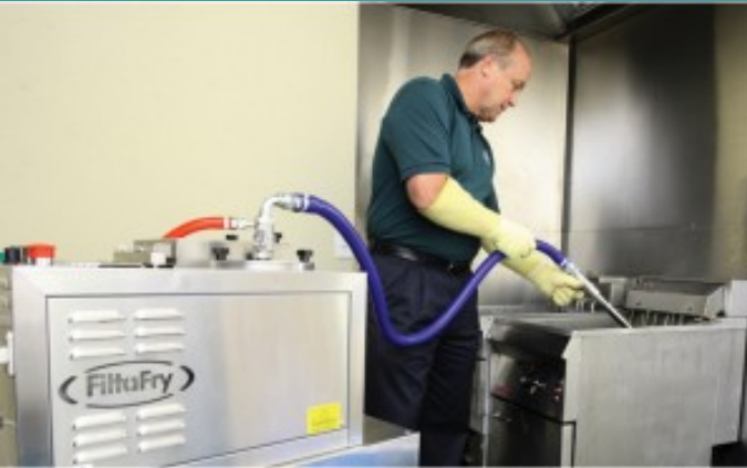
Removing oil from fryer and filter
